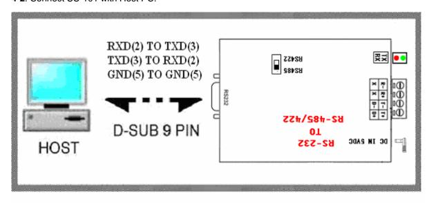
4-3. Connect SC-485 with RS4222 or RS422/485 serial device.
