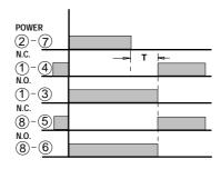
COM. : Common terminal N.C. : Normally closed contact N.O. : Normally open contact  $\bigcirc \bigvee \bigcirc$  : Off time out contact
