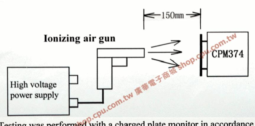
Testing was performed with a charged plate monitor in accordance with Ionization Standard ANSI/ESD STM3.1-2000 of the ESD Association.
