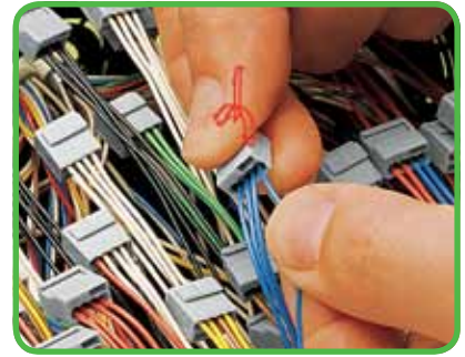
Removal Hold wire to be removed and twist alternating left and right while pulling the conductor
