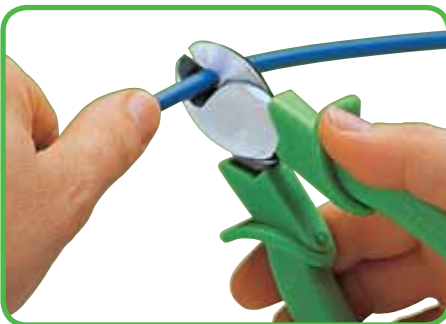
Cutting of wire
