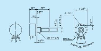
Note: 1. 1 pc. each inner teeth washer and hex nut are attached.
