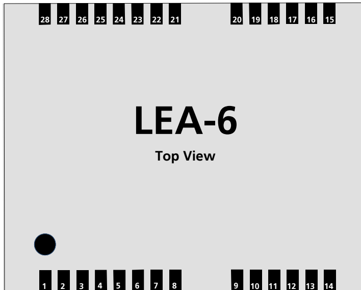
Figure 2 LEA-6 Pin Assignment
