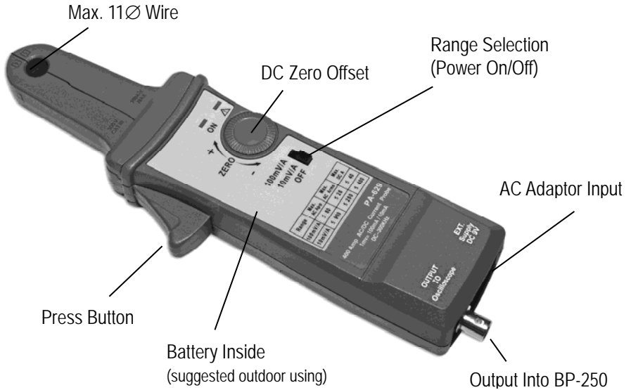
Figure 1: shows the controls and indicators on the PA-659 current probe.
