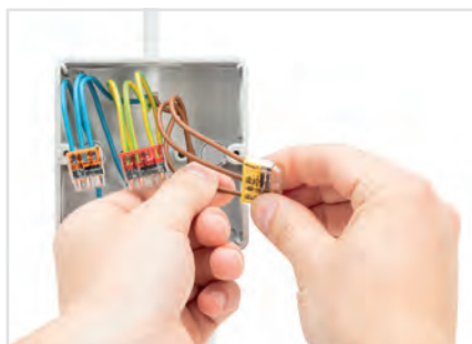
Removal: Hold solid conductor to be removed and twist alternately left and right while pulling the connector. Stranded wire: simply cut the wire close to the connector entry, strip it and insert into a new connector.
