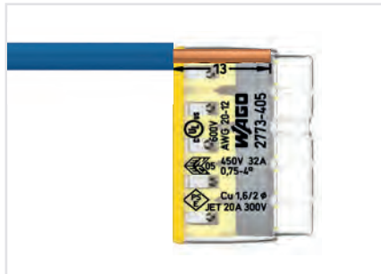
Strip solid or stranded conductor to 13 mm (0.51 inch).
